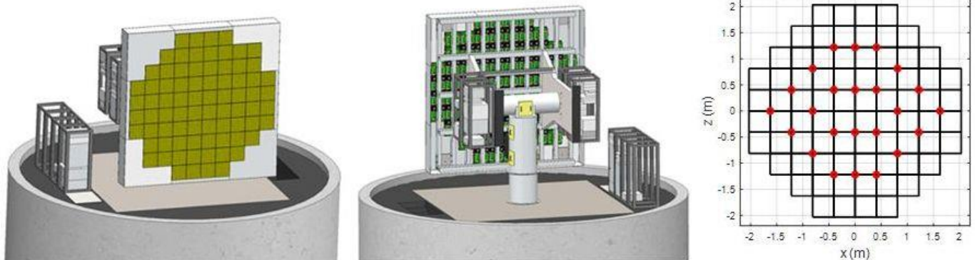
Figure 2.1.1. Front (left panel) and back (middle panel) of the antenna assembly. The antenna layout with subarray centers shown as red dots (right panel).
